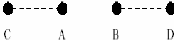
Fig. 2. Neighboring nodes A and B have different schedules. They synchronize with nodes C and D respectively.
