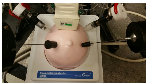
Figure 5. Schematic setup using four external vibration sources to generate a reverberation field inside the breast tissue mimicking phantom.
