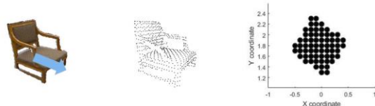
Figure 3. An example of using entity model to describe a chair. LEFT: the chair sample (The arrow illustrates its direction); MIDDLE: the 3-D point cloud of the chair; RIGHT: the 2-D point cluster \rho . The direction angle is 4\pi/7 rad (or 315^\circ ). The entity model e = \{ \text{"chair"}, \rho, 7/4\pi \} .
