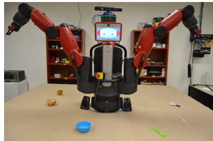
Fig. 1. The experimental setup from the participant’s perspective: a Baxter robot has six objects within reach. The participant stands in front of the table to provide speech and gesture requests
