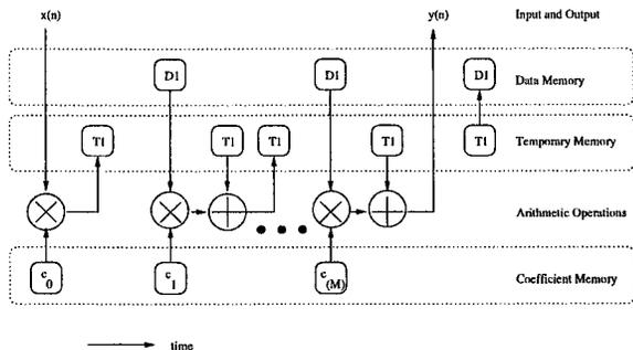
Figure 2: Register transfer level representation of a FIR filter.
