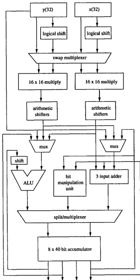
Figure 4: Simplified Lucent Technologies DSP16xxx data path.
