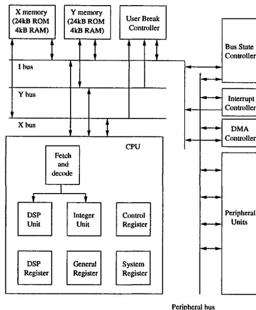
Figure 9: Simplified SH-DSP family processor architecture.
