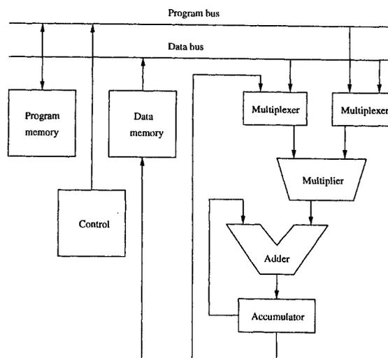
Figure 3: First generation conventional DSP architecture.
