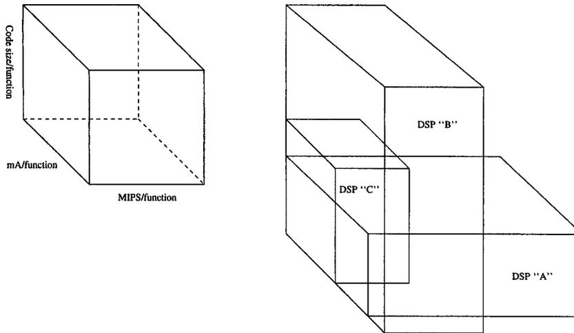
Evaluating three different DSP processors for a modem application
