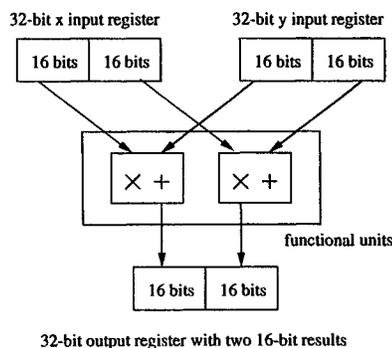
Figure 5: SIMD split execution unit data path.
