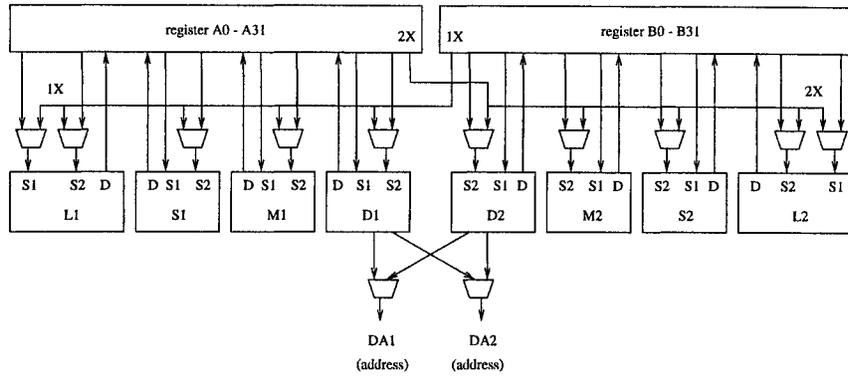
Figure 7: Simplified diagram of the 'C64x data cross paths.
