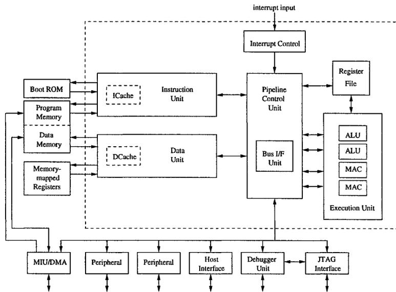
Figure 8: ZSP16400 processor architecture.
