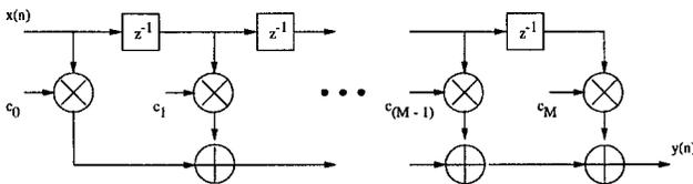
Figure 1: Tapped delay line structure of a FIR filter.
