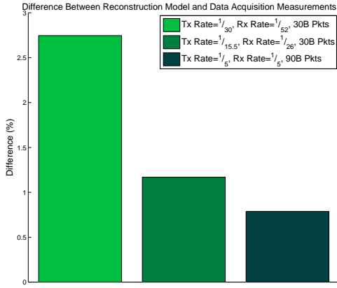
Fig. 2. Relative difference between real life scenarios and their prediction through the reconstruction model for various values of the rates of sent and received packets.
