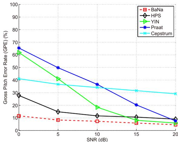
Figure 3.15: GPE rate of the different algorithms for a piece of clarinet music with eight types of noise. Detected  $F_0$  deviating more than 3% from ground truth are errors.
