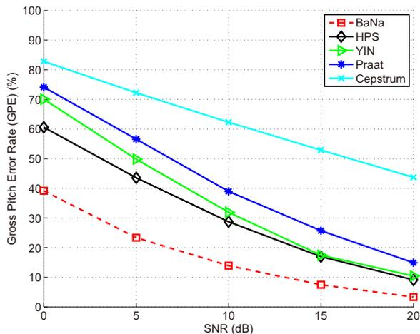
Figure 3.16: GPE rate of the different algorithms for a piece of piano music with eight types of noise. Detected  $F_0$  deviating more than 3% from ground truth are errors.
