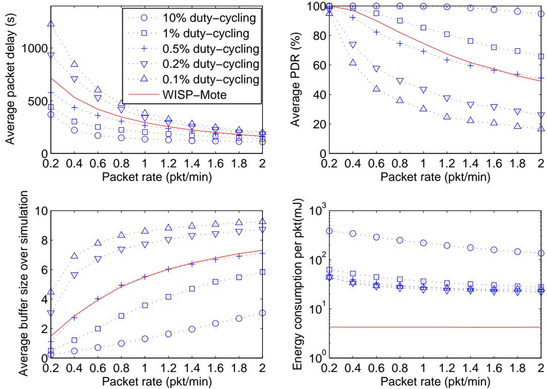
Figure 2.9: WISP-Mote vs. duty-cycling with limited buffer size ( $0.002 \text{ nodes}/m^2$ , 1 data MULE, buffer size = 10 *pkts*).
