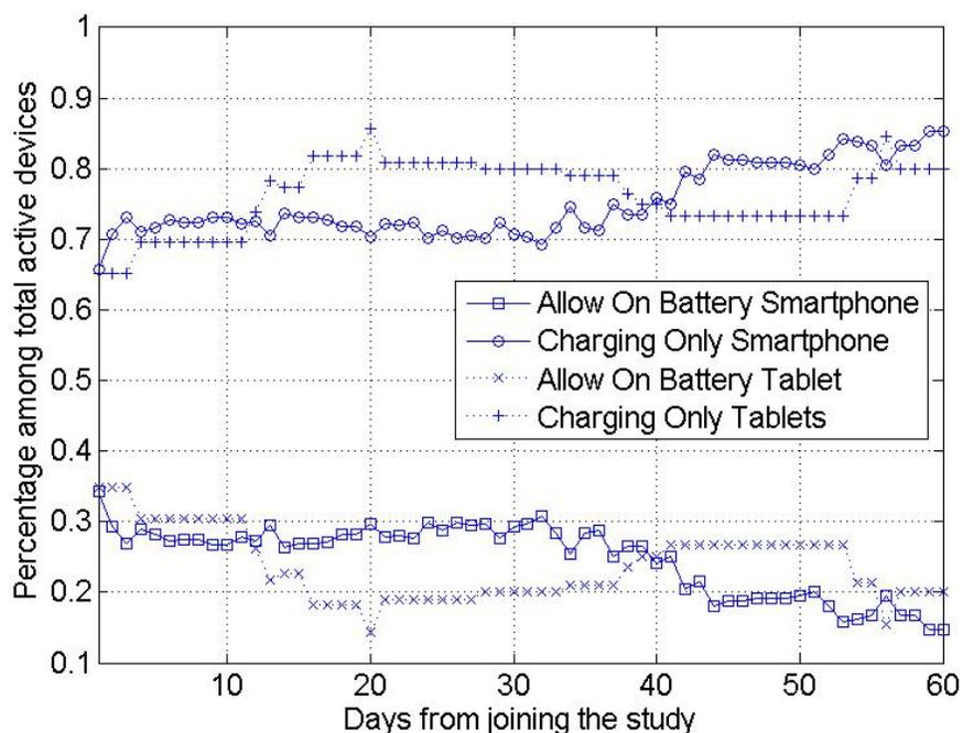
Figure 6.13: Number of devices that allow computing on battery vs. charging only.
