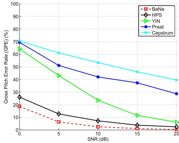
Figure 3.14: GPE rate of the different algorithms for a piece of trumpet music with eight types of noise. Detected  $F_0$  deviating more than 3% from ground truth are errors.
