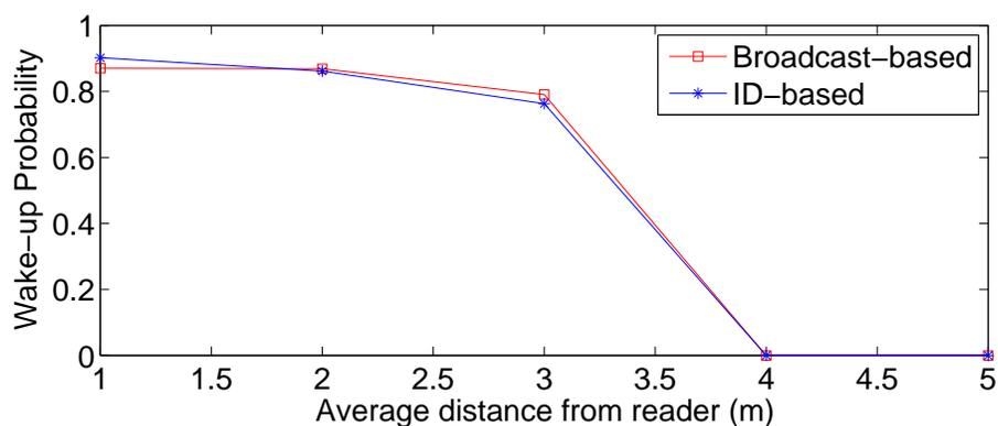
Figure 2.6: Broadcast-based wake-up and ID-based wake-up probabilities in a clustered environment.
