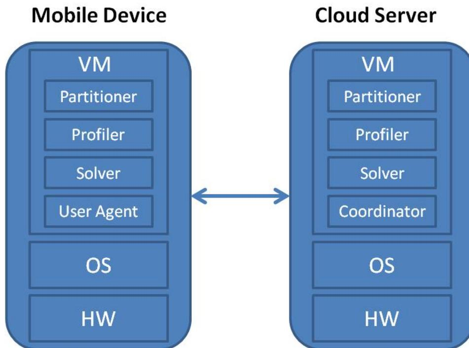
Figure 4.1: A generalized mobile-cloud architecture.
