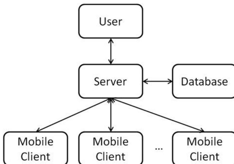
Figure 5.2: The mobile computing system architecture.
