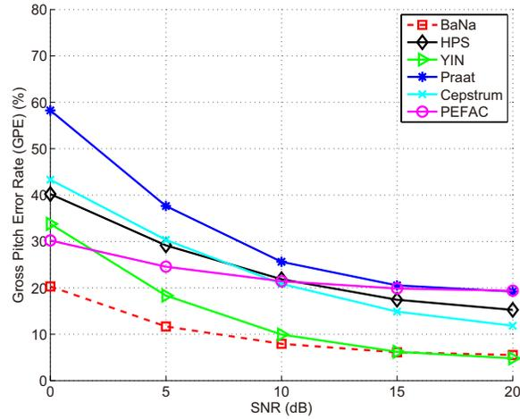
Figure 3.7: GPE rate of the different algorithms for the KEELE database [5], averaged over all eight types of noise. Detected  $F_0$  deviating more than 10% from ground truth are errors.
