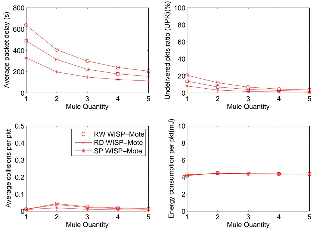
Figure 2.11: Comparisons among different mobility models for the data MULE; RW=Random Walk, RD=Random Direction, SP=Snake Path ( $0.002 \text{ nodes}/m^2$ ,  $1 \text{ pkt}/min$ , unlimited buffer size).
