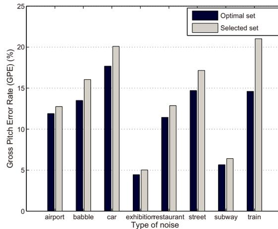
Figure 3.4: GPE rates of BaNa for the LDC database [2] with eight types of AURORA noise [3] averaged over all SNR values, using individually optimized parameter sets that provide the lowest GPE rates for a specific type of AURORA noise, and using the tuned parameter set selected in the chapter. Detected  $F_0$  deviating more than 10% from ground truth are errors.
