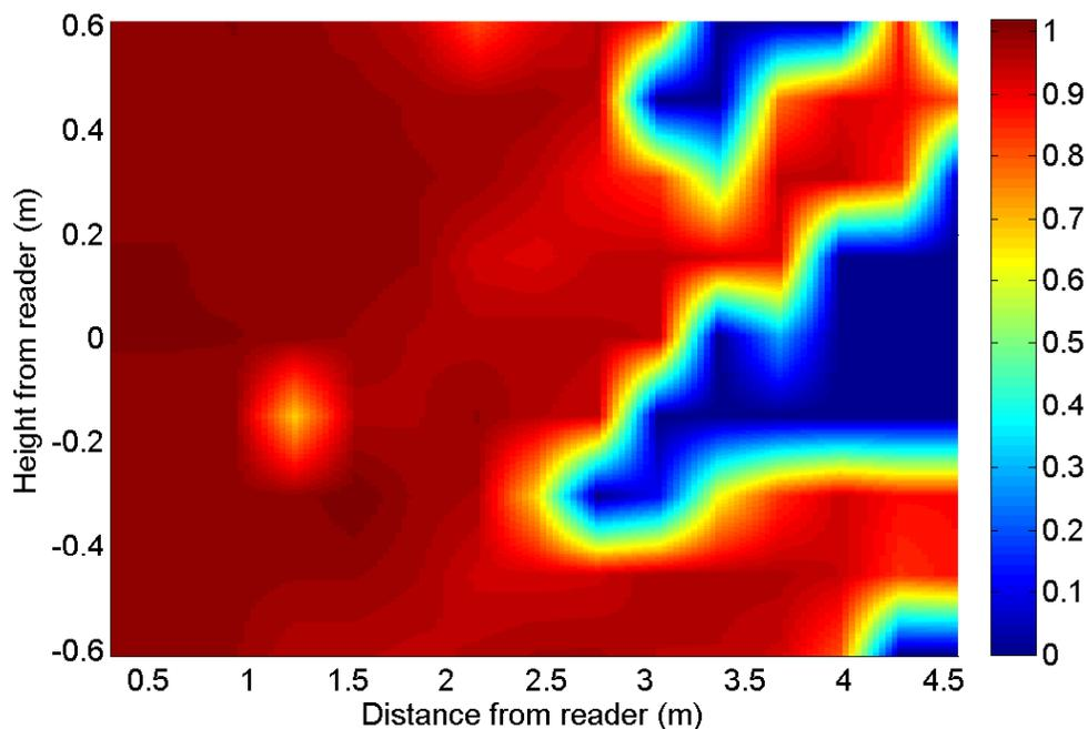
Figure 2.2: Broadcast-based wake-up probabilities in an open environment.
