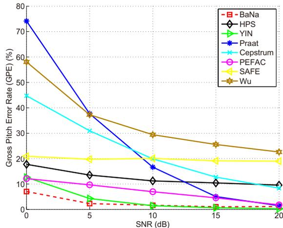
Figure 3.9: GPE rate of the different algorithms for the LDC database [2] for speech with white noise. Detected  $F_0$  deviating more than 10% from ground truth are errors.
