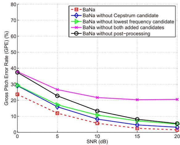
Figure 3.11: GPE rate of BaNa, BaNa without the Cepstrum candidate, BaNa without the lowest frequency candidate, BaNa without both added candidates, and BaNa without post-processing for the LDC database, averaged over all eight types of noise. Detected  $F_0$  deviating more than 10% from ground truth are errors.
