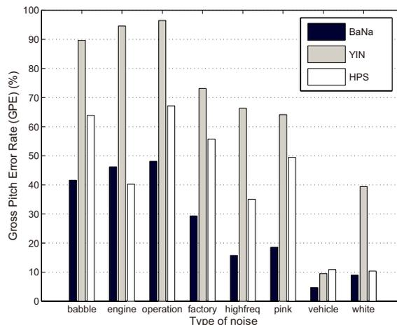
Figure 3.17: GPE rate of BaNa, YIN and HPS for a piece of violin music with eight types of noise at 0 dB SNR. Detected  $F_0$  deviating more than 3% from ground truth are errors.
