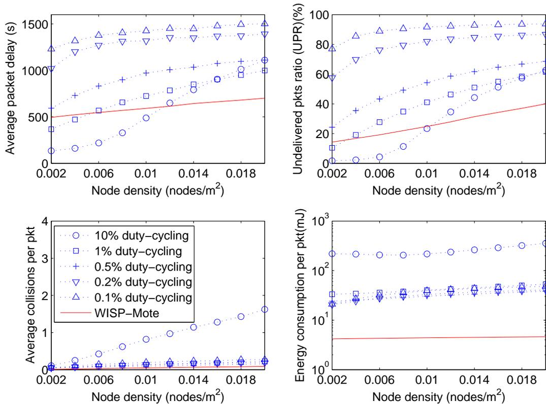
Figure 2.8: WISP-Mote vs. duty-cycling with increasing node density (1 *pkt/min*, 1 data MULE, unlimited buffer).
