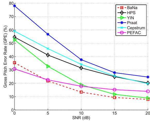
Figure 3.6: GPE rate of the different algorithms for the CSTR database [4], averaged over all eight types of noise. Detected  $F_0$  deviating more than 10% from ground truth are errors.
