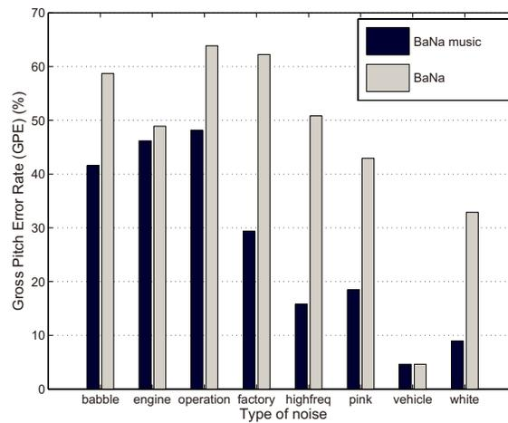
Figure 3.12: GPE rate of BaNa and BaNa music for a piece of violin music with eight types of noise at 0 dB SNR. Detected  $F_0$  deviating more than 3% from ground truth are errors.
