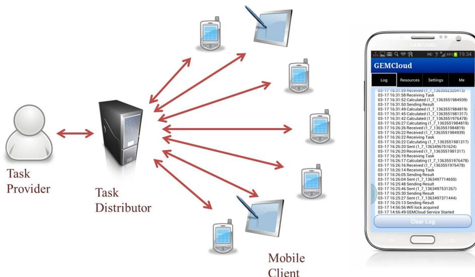
Figure 6.1: The architecture of the GEMCloud platform.
