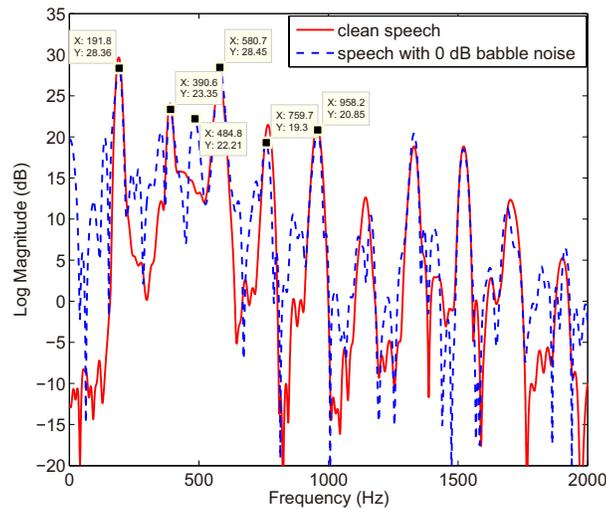
Figure 3.1: Spectrum of one frame of clean speech and speech with babble noise at 0 dB SNR.
