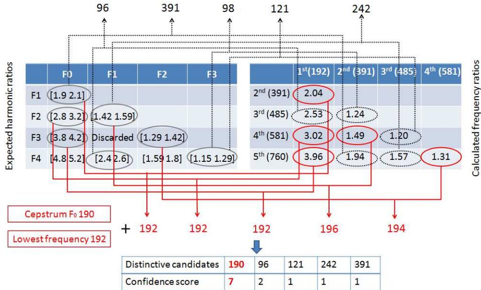
Figure 3.2: Tolerance ranges for harmonic ratios when the number  $p$  of selected spectral peaks is set to 5, and an example to illustrate the procedure for determining the  $F_0$  candidates.
