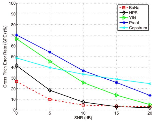
Figure 3.13: GPE rate of the different algorithms for a piece of violin music with eight types of noise. Detected  $F_0$  deviating more than 3% from ground truth are errors.
