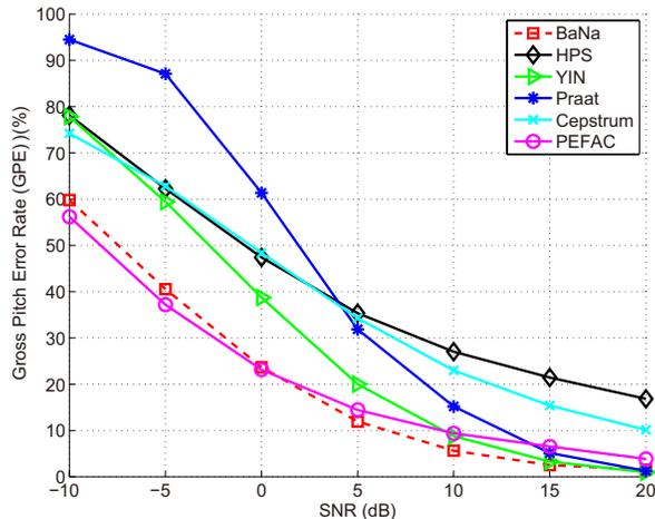
Figure 3.5: GPE rate of the different algorithms for the LDC database [2], averaged over all eight types of noise. Detected  $F_0$  deviating more than 10% from ground truth are errors.
