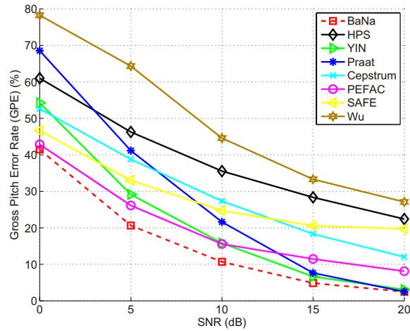
Figure 3.8: GPE rate of the different algorithms for the LDC database [2] for speech with babble noise. Detected  $F_0$  deviating more than 10% from ground truth are errors.
