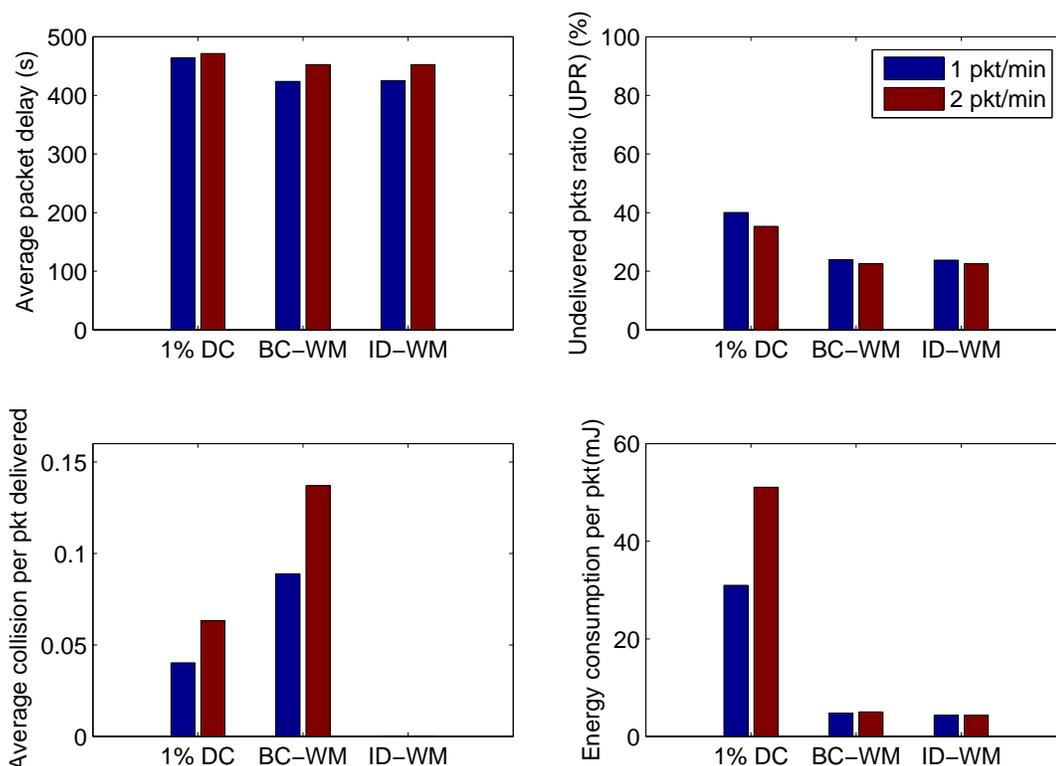
Figure 2.12: Patient monitoring scenario (unlimited buffer), “BCWM stands for Broadcast-based WISP-Mote, “ID-WM stands for ID-based WISP-Mote.
