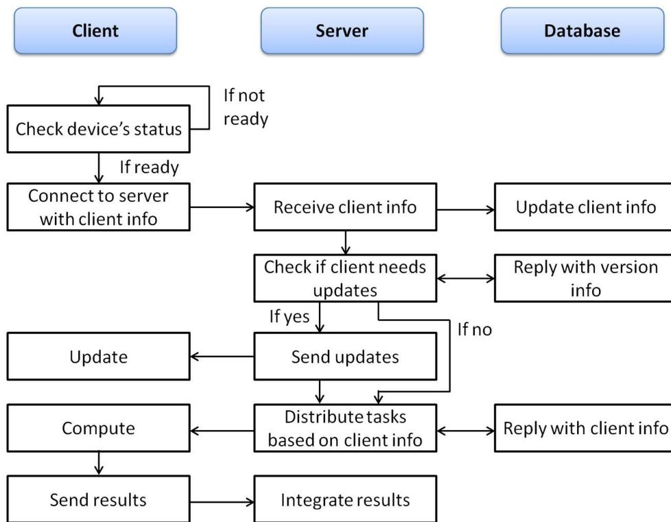
Figure 5.3: The server-client protocol flow chart.
