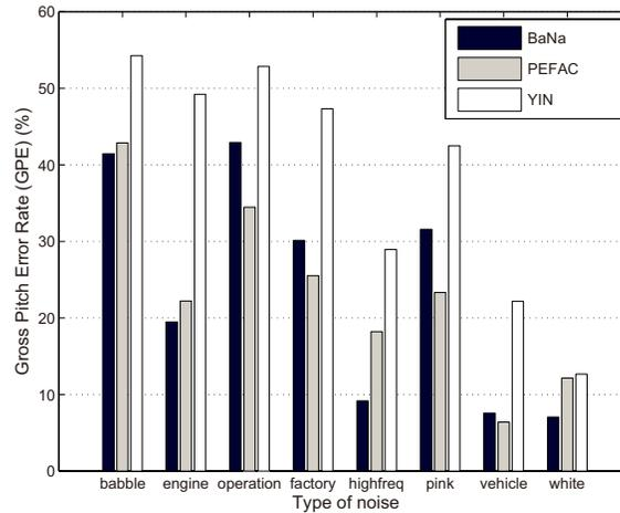
Figure 3.10: GPE rate of BaNa, PEFAC and YIN for the LDC database [2] with eight types of noise at 0 dB SNR. Detected  $F_0$  deviating more than 10% from ground truth are errors.
