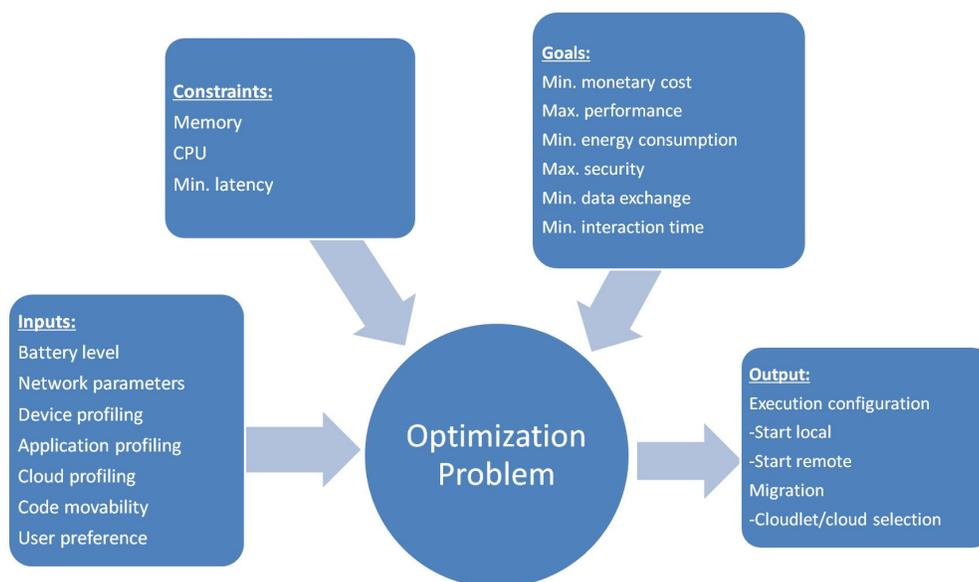
Figure 4.3: The cost model of mobile cloud computing (adapted from [7,8]).
