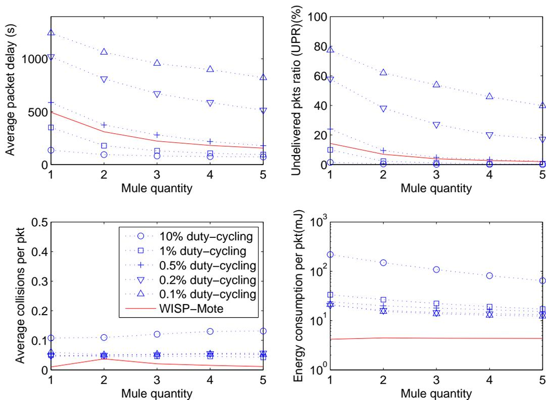
Figure 2.10: WISP-Mote vs. duty-cycling with increasing MULE quantities ( $0.002 \text{ nodes}/\text{m}^2$ ,  $1 \text{ pkt}/\text{min}$ , unlimited buffer size).
