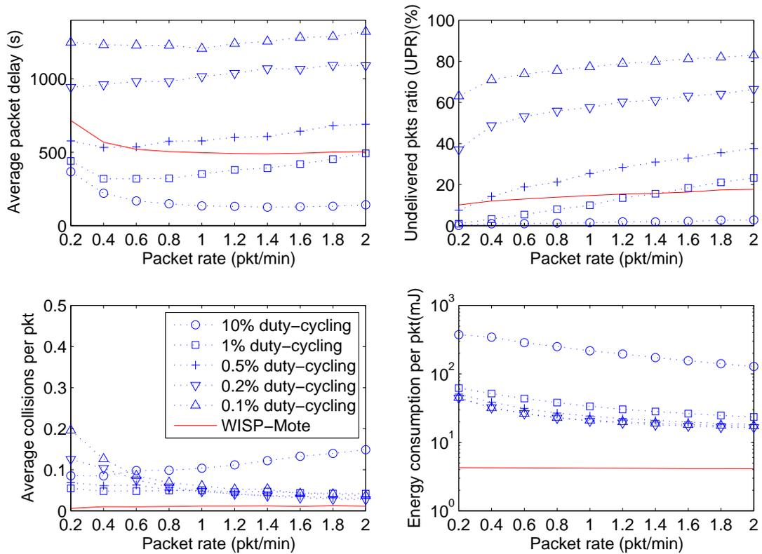
Figure 2.7: WISP-Mote vs. duty-cycling with increasing packet rate ( $0.002 \text{ nodes}/m^2$ , 1 data MULE, unlimited buffer).
