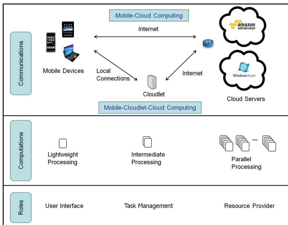
Figure 4.2: The Mobile-Cloud computing and Mobile-Cloudlet-Cloud computing architectures: mobile devices directly interact with a cloud or via the cloudlet and use dynamic partitioning to achieve their quality of service (QoS) goals (e.g., latency, cost).
