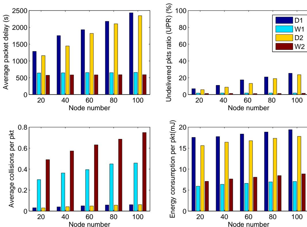
Figure 2.13: Animal monitoring scenario; D1= 1% Duty-cycling with  $R = 1$ , W1=WISP-Mote with  $R = 1$ , D2=1% Duty-cycling with  $R = 2$ , W2=WISP-Mote with  $R = 2$  ( $0.2 \text{ pkt}/\text{min}$ , buffer size unlimited)
