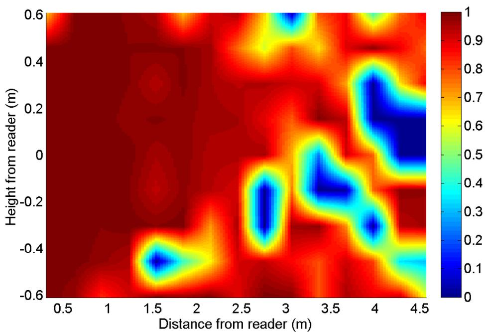
Figure 2.4: Broadcast-based wake-up probabilities in a closed environment.
