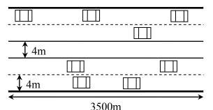
Figure 2: Highway scenario: a model Highways are modeled as two groups of straight lanes of size *numLanes* x 4m by 3500m, separated by 4m.
