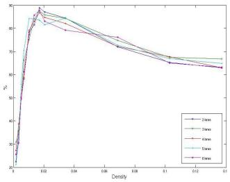
Figure 6: Average PDR vs. Density for 2-to-6 lane bidirectional highways. The number of lanes on the highway does not affect the behavior of the average PDR. The average number of delivered packets peaks at a density between 0.017 and 0.021.
