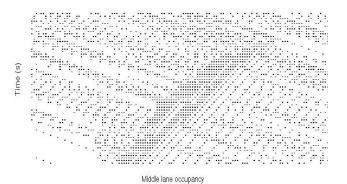
Figure 4: Backward movement on a 5-lane highway On each lane of the highway (here: middle lane), the traffic jam goes backward over the 60s of our simulated traffic.
