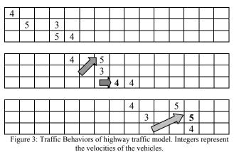
Cars traveling on the highway look for alternate paths when there is an obstacle ahead. If a car cannot find an alternate route, it slows down and reaccelerates when the traffic allows.
