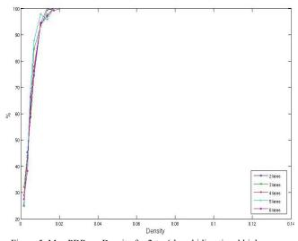
Figure 5: Max PDR vs. Density for 2-to-6 lane bidirectional highways. All nodes receive at least one notification packet for a density of at least 0.017.
