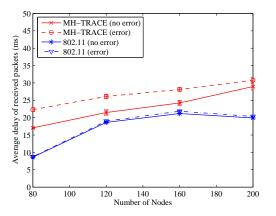
Fig. 12. SET 2 (mobile nodes): Average data packet delay versus number of nodes.
