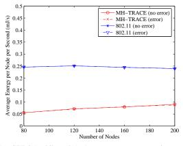
Fig. 11. SET 2 (mobile nodes): Average energy consumption per node per second versus number of nodes.
