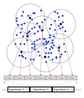
Fig. 2. A snapshot of MH-TRACE clustering and medium access for a portion of an actual distribution of mobile nodes. Nodes  $C_1$  -  $C_7$  are clusterhead nodes.
