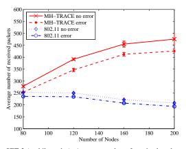
Fig. 8. SET 2 (mobile nodes): Average number of received packets per node per second versus number of nodes.
