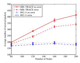
Fig. 7. SET 1 (stationary nodes): Average number of received packets per node per second versus number of nodes.
