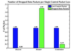
Fig. 4. MH-TRACE performance degradation in terms of dropped data packets for beacon, header, and contention packet losses.
