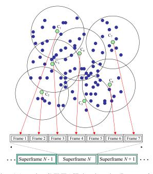
Figure 1. A snapshot of MH-TRACE clustering and medium access for a portion of an actual distribution of mobile nodes. Nodes  $C_1$  -  $C_7$  are CHs.
