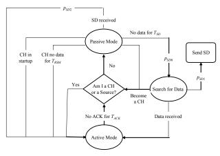
Figure 3. NB-TRACE flowchart.
