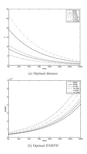
Figure 4.3: Energy optimal hop distance as a function of noise.  $E_{s,TX} = 5x10^{-9}J$ .
