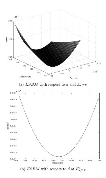
Figure 4.2: Demonstrating optimal hop distance.
