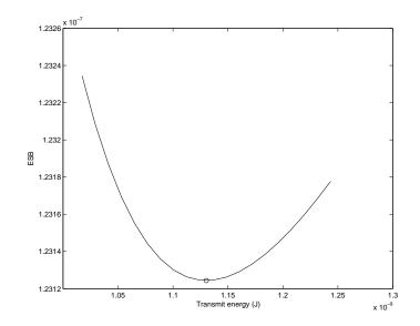
Figure 3.2: The ESB as a function of the transmit energy  $E_{s,TX}$ . This plot shows a clear minimum and thus the optimal transmit energy. These results assume a fixed distance d = 10m, BPSK modulation and fixed channel noise.
