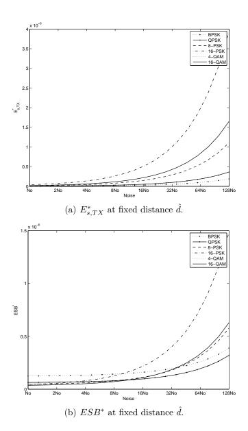
Figure 4.1:  $E_{s,TX}^*$  and  $ESB^*$  for a fixed distance,  $\hat{d} = 15m$  at a range of noise values for different modulations.
