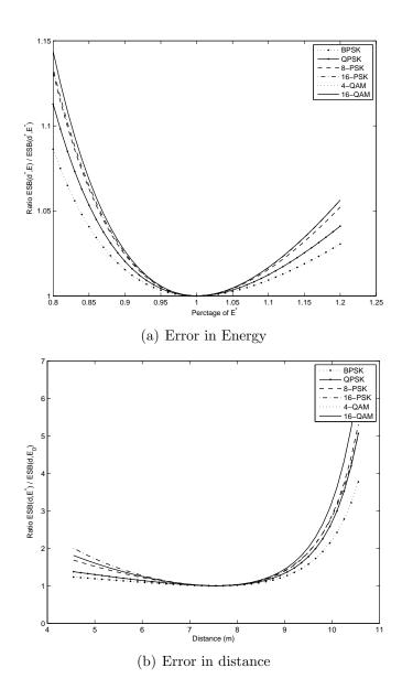
Figure 4.9: Gain of finding optimal transmit energy and optimal distance.
