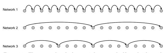
Figure 1.1: Three examples of a linear wireless network. Network 1 has a short hop distance, Network 2 has a long hop distance, and Network 3 has the optimal hop distance.
