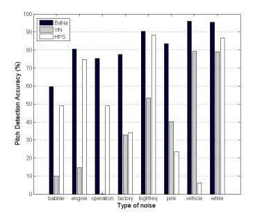
Figure 3.16: Pitch detection accuracy of BaNa, YIN and HPS for a piece of trumpet music with eight types of noise at 0dB.
