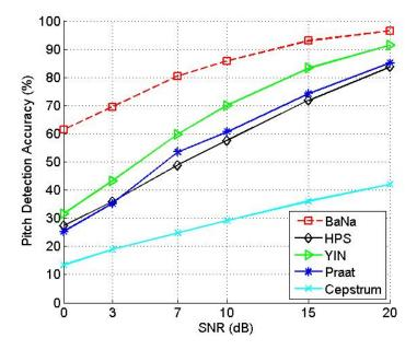
Figure 3.14: Pitch detection accuracy of the different algorithms for a piece of slow tempo piano music.
