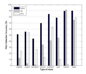
Figure 3.17: Pitch detection accuracy of BaNa, YIN and HPS for a piece of violin music with eight types of noise at 0dB.
