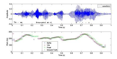
Figure 3.1: Speech waveform and the auto-labeled ground truth derived from three algorithms for one speech utterance.
