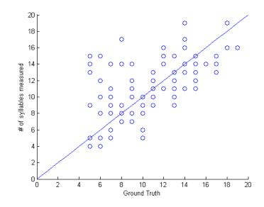
Figure 3.23: Scatter plots of detected syllable numbers versus the ground truth for the 100 utterances corrupted with 0dB white noise. Hybrid estimator.
