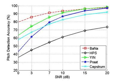
Figure 3.4: Pitch detection accuracy of the different algorithms for the Harvard Sentences database.
