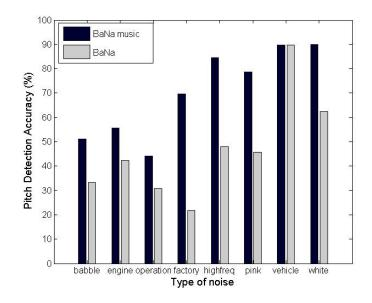
Figure 3.9: Pitch detection accuracy of BaNa and BaNa music for a piece of violin music with eight types of noise at 0dB.
