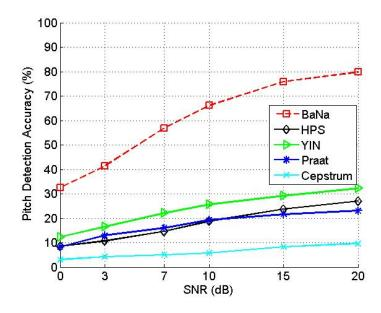
Figure 3.13: Pitch detection accuracy of the different algorithms for a piece of fast tempo piano music.
