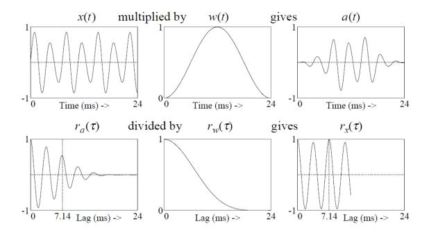
Figure 2.3: Flowchart of the Praat algorithm, reprinted from [3].
