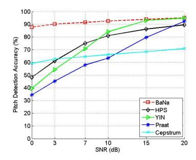
Figure 3.10: Pitch detection accuracy of the different algorithms for a piece of clarinet music.
