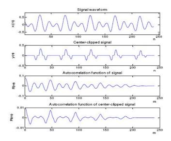
Figure 2.2: An illustration of the effect of center clipping, reprinted from [2].
