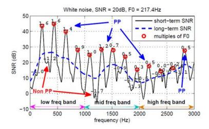
Figure 2.7: The SNR spectrum for white noise SNR-20dB, *F*0=217.4Hz, reprinted from [6].
