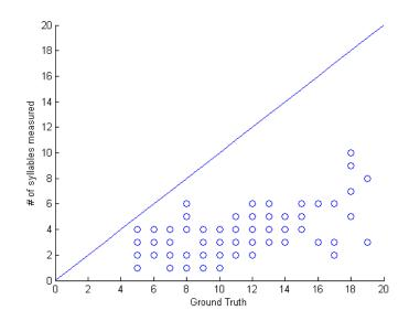
Figure 3.20: Scatter plots of detected syllable numbers versus the ground truth for the 100 utterances corrupted with 0dB white noise. Full band estimator.
