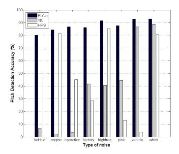
Figure 3.15: Pitch detection accuracy of BaNa, YIN and HPS for a piece of clarinet music with eight types of noise at 0dB.
