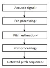
Figure 2.1: The work flow of a typical pitch estimation algorithm.
