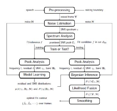
Figure 2.6: Flowchart of the SAFE algorithm, reprinted from [6].
