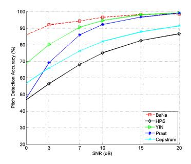
Figure 3.3: Pitch detection accuracy of the different algorithms for the Arctic database.
