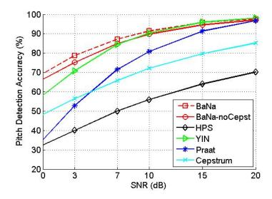
Figure 3.2: Pitch detection accuracy of the different algorithms for the LDC database.
