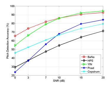
Figure 3.5: Pitch detection accuracy of the different algorithms for the CSTR database.
