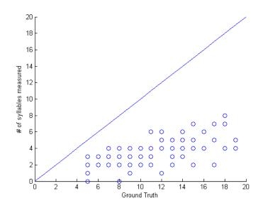
Figure 3.21: Scatter plots of detected syllable numbers versus the ground truth for the 100 utterances corrupted with 0dB white noise. Sub-band M=4 estimator.
