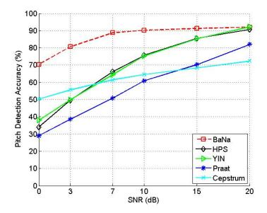
Figure 3.12: Pitch detection accuracy of the different algorithms for a piece of violin music.
