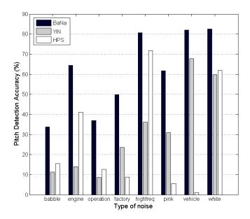
Figure 3.19: Pitch detection accuracy of BaNa, YIN and HPS for a piece of slow tempo piano music with eight types of noise at 0dB.
