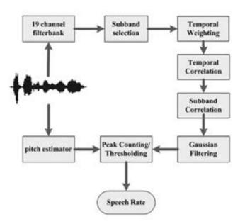
Figure 2.10: Flowchart of the hybrid speaking rate estimator, reprinted from [7]. the energy in each time frame is recalculated using the following equation,
