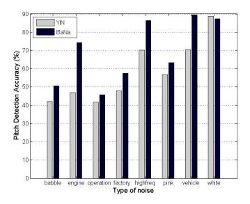
Figure 3.6: Pitch detection accuracy of BaNa and YIN for the LDC database with eight types of noise at 0dB.
