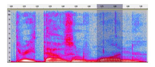
Figure 2.8: Spectrogram of an utterance "Three thousand one."
