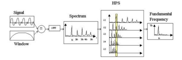
Figure 2.4: Flowchart of the HPS algorithm, reprinted from [4].
