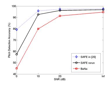
Figure 3.7: Pitch detection accuracy of BaNa and SAFE for the CSTR database [8] for speech with babble noise.
