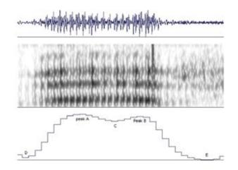
Figure 2.9: The waveform, spectrogram and the energy envelop of an utterance "Bad." Illustration of a case that a single syllable displays two peaks, reprinted from [7].
