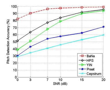
Figure 3.11: Pitch detection accuracy of the different algorithms for a piece of trumpet music.
