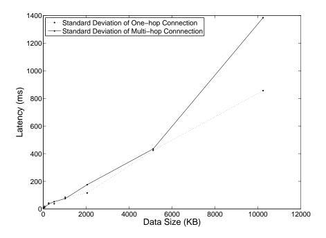
Figure 4.5: Standard deviations of communication latency via single hop and multi-hop WiFi connections.
