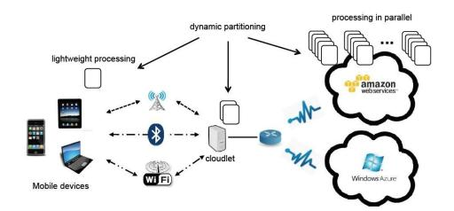
Figure 2.1: The MOCHA architecture: mobile devices interact with the cloudlet and the cloud via multiple connections and use dynamic partitioning to achieve their QoS goals (e.g., latency, cost) (reprinted from (Soyata, T., Muraleedharan, R., Funai, C., Kwon, M., & Heinzelman, W., 2012) with permission of the authors).
