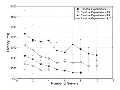
Figure 5.5: Experiment: the random algorithm with 1, 3, 5 and 10 redundant copies of the data sent to the same number of servers. Given our overall limited number of servers, at a redundance of R = 10, we do not have enough servers to split the data into more than 4 chunks (which translates to 40 servers). Here, data size M=1024 (KB), total number of servers =41 (41 of 55 nodes with valid data).
