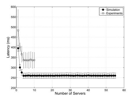
Figure 5.7: Simulation and experiment results for the greedy algorithm as we increase N, the number of servers considered for sending data. In this algorithm, each server receives a different amount of data depending on what data size at that server minimizes latency. Here, data size M=1024 (KB).
