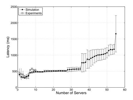
Figure 5.6: Simulation and experiment results for the fixed algorithm as we increase N, the number of servers considered for sending data. In this algorithm, each server receives  $\lceil \frac{M}{N} \rceil$  amount of data. Here, data size M=1024 (KB).
