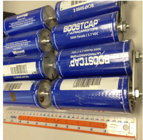
Fig. 3. Energy buffer: 8 series Maxwell BCAP3000 supercapacitors [17].
